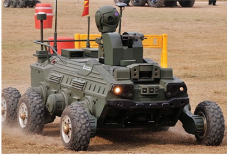
Fig. 5. 6 × 6 unmanned robot vehicle.
