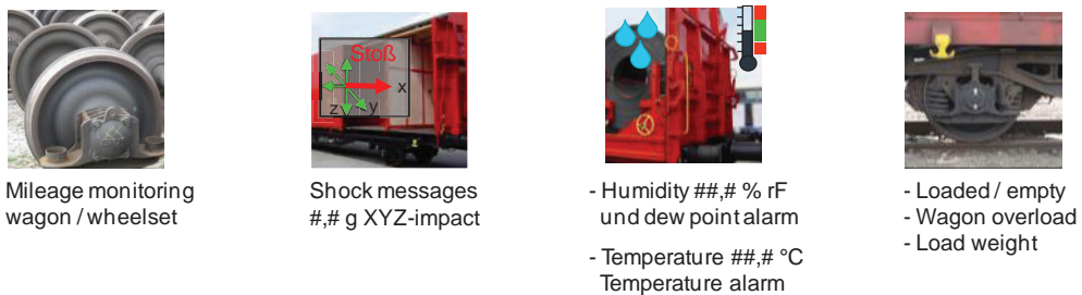
Fig. 6. Telematics extended with condition monitoring functionality (source: Eureka).
