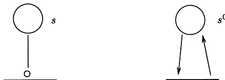
Fig. 4. An inhibiting arc on place s of a primitive system is represented as a self-loop on place s^0 in the corresponding P/T system.
