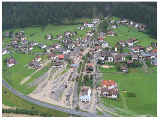
Fig. 2. The event of 22 August 2005, classified as a fluvial sediment transport process, at the Schnannerbach torrent in the municipality of Pettneu am Arlberg (courtesy of ASI Tirol).
