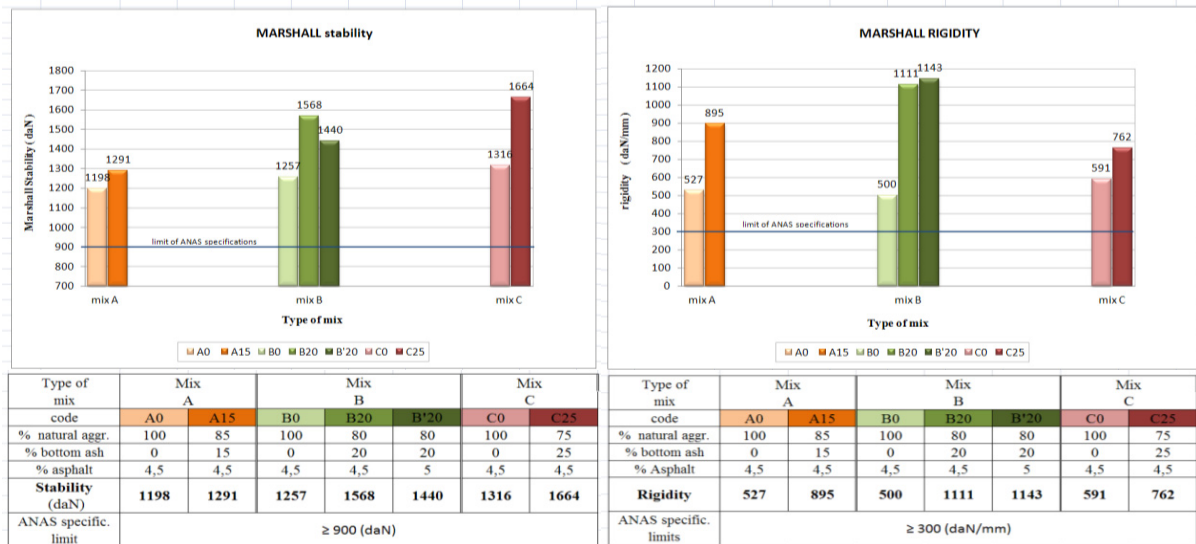
Fig. 7. (a) Marshall stability results; (b) Marshall rigidity
