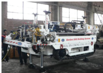
Figure 8 VLD1000 type drilling system of Valley Longwall International Group Companie
