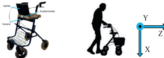
Fig. 1. (a) Hardware setup; (b) Accelerometer axis configuration.
