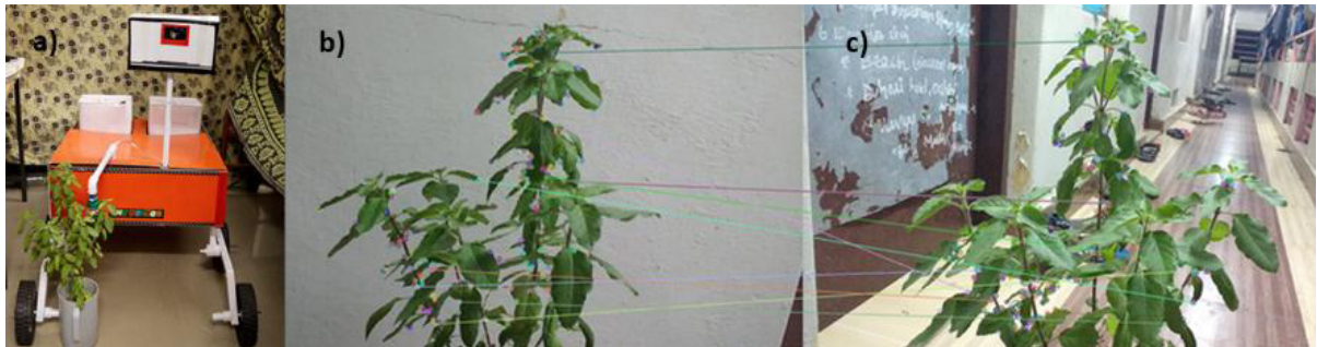
Fig.5. (a) Smart autonomous gardening rover (ALIVE); (b) Feature extracted plant image; (c) Real-time plant image matched using FLANN matcher
