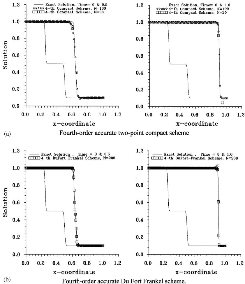
Fig. 2. The computed solutions of one-dimensional unsteady Burgers' equation, for  $\nu = 0.001$  and at times = 0.5 and 1.0, using compact scheme with two-grid sizes  $N = 20$  and 100, and Du Fort Frankel scheme with  $N = 200$ : (a) fourth-order accurate two-point compact scheme and (b) fourth-order accurate Du Fort Frankel scheme.
