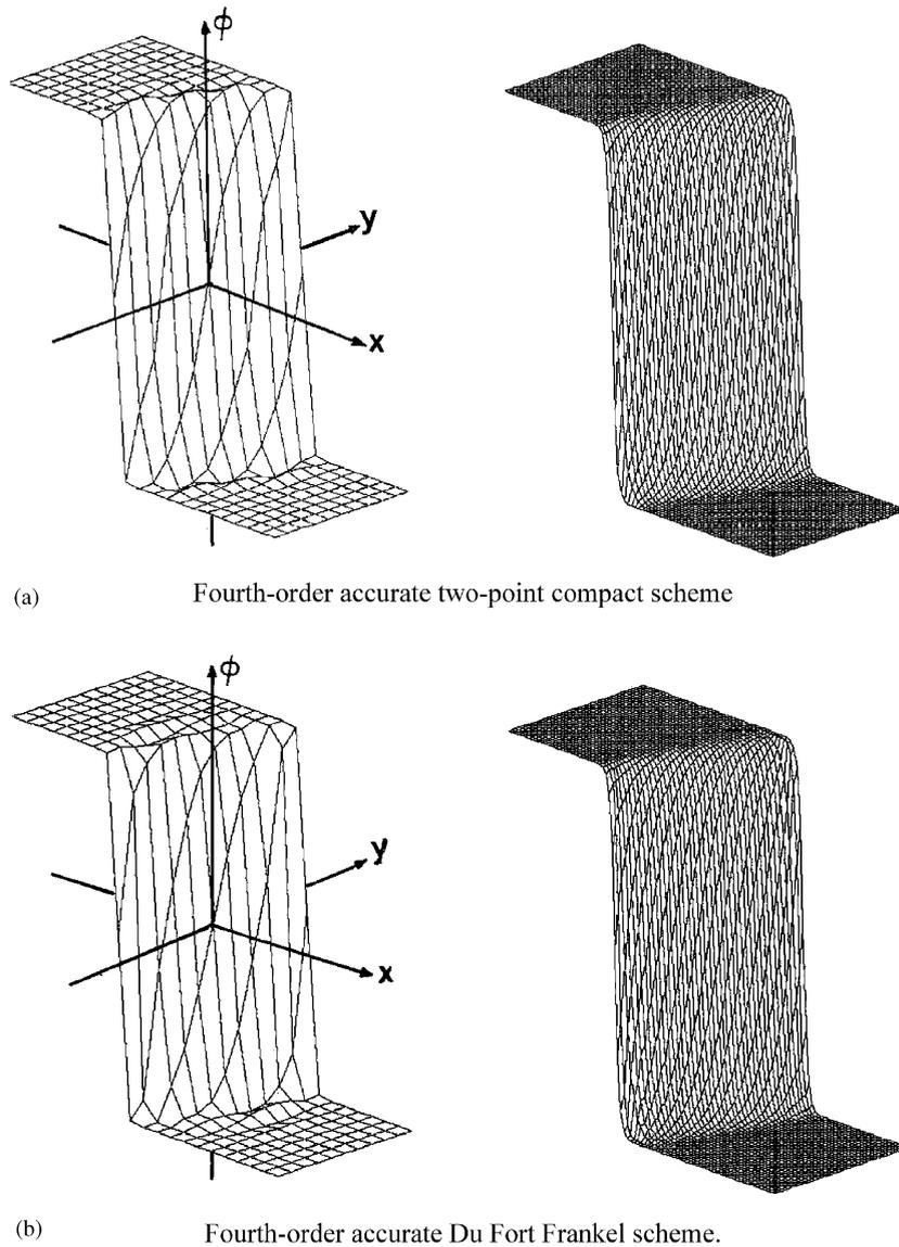
Fig. 5. The computed steady state solutions of two-dimensional unsteady Burgers' equation for an oblique shock case, with  $\nu = 0.002$ , for two different grid sizes;  $(80 \times 40)$  &  $(20 \times 10)$ , using compact scheme and Du Fort Frankel scheme: (a) fourth-order accurate two-point compact scheme and (b) fourth-order accurate Du Fort Frankel scheme.
