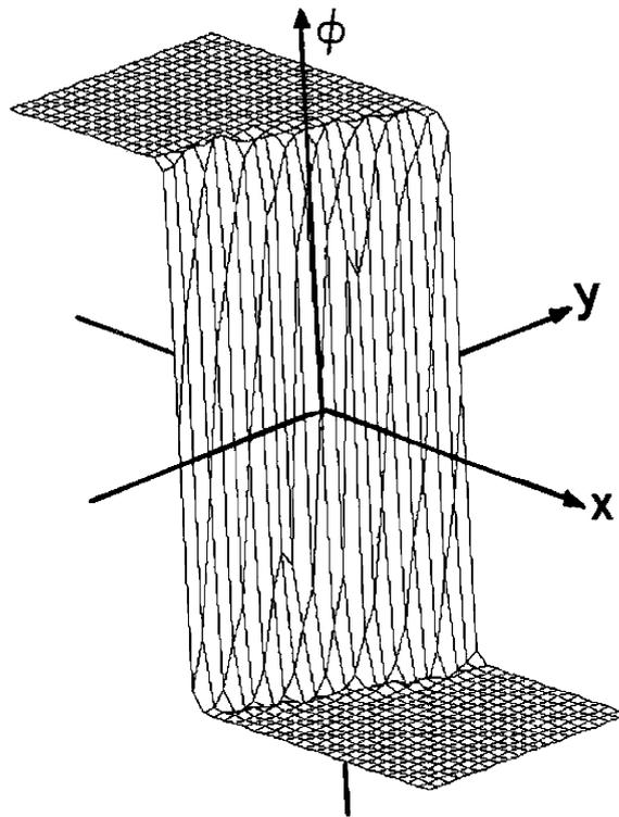
Fig. 6. The computed steady state solutions of two-dimensional unsteady Burgers' equation for an oblique shock case, with  $\nu = 0.0005$  and grid size  $(40 \times 20)$ , using the fourth-order accurate compact scheme.
