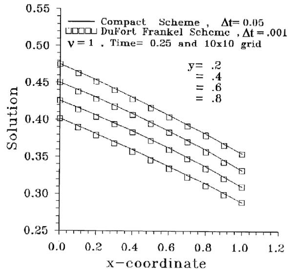
Fig. 3. The computed steady state solutions of two-dimensional unsteady Burgers' equation for test case 2, using compact scheme with  $\Delta t = 0.05$  and their comparison with Du Fort Frankel scheme with  $\Delta t = 0.001$ .
