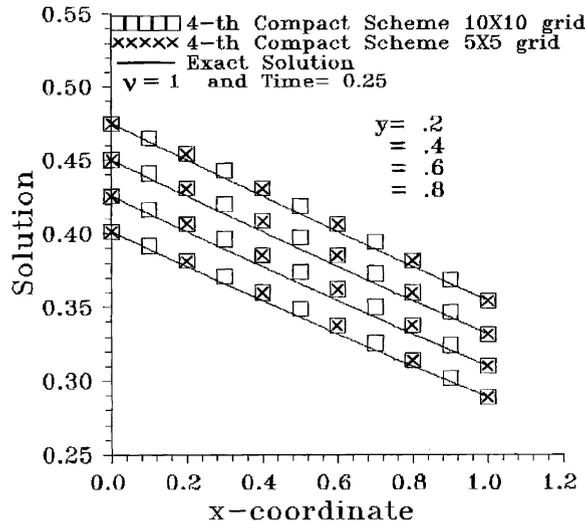
Fig. 4. The computed steady state solutions of two-dimensional unsteady Burgers' equation for test case 2, using compact scheme with different grid sizes, and their comparison with the exact solutions.
