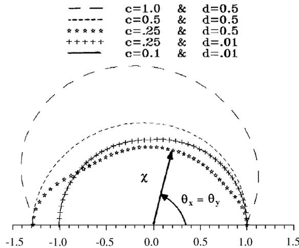
Fig. 1. The computed amplification factors of the numerical solution of two-dimensional unsteady Burgers' equation (1), using the explicit fourth-order Du Fort Frankel scheme for different values of  $|c|$  and  $d$ .
