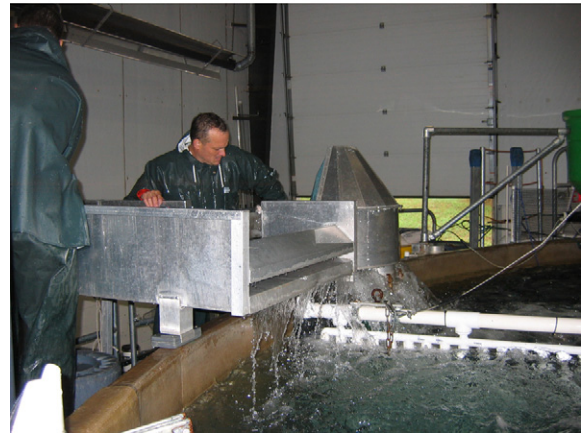
Fig. 8. Picture showing the stationary grader gate of the clam-shell crowder/grader (in bottom photo; note, gates used to pivot about the tank are not shown) and the airlift pump and dewatering box that is placed above and to one side of the culture tank, resting on the tank's lip. The clam-shell crowder/grader and the airlift pump and hand sorting/dewatering box were used in combination to selectively harvest Arctic char and rainbow trout (shown) from the 150 m 3 growout tank.
