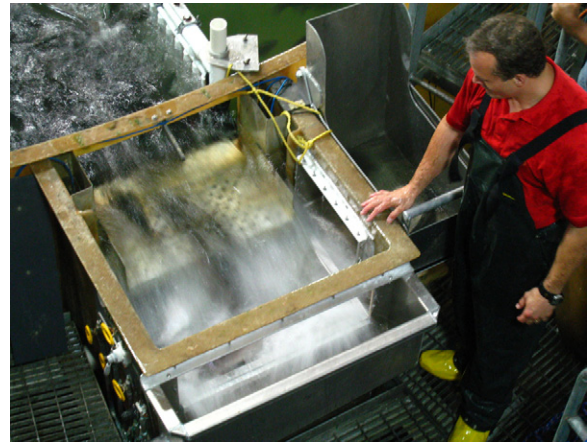
Fig. 16. The normally vertical and perforated door through the sidewall drain has been lowered and fish crowded to this location are rapidly flowing onto a dewatering rack. The fish pass over the dewatering rack and into the primary outlet channel box, which is located opposite the entry gate. Smaller fish can be hand-sorted while above the dewatering rack and slid into a secondary outlet box (pictured on the right hand side), which contains a screened basket that is hinged to allow fish placed in the box to slide back into the culture tank when the basket is lifted up, i.e., pivoting its lower lip over the culture tank, just to the outside of the clam-shell crowder. The primary outlet chamber slopes more than 5% to its lower end, where it connects to a 20-cm diameter transfer hose (not shown); the transfer hose is used to slide harvested fish to another location.
