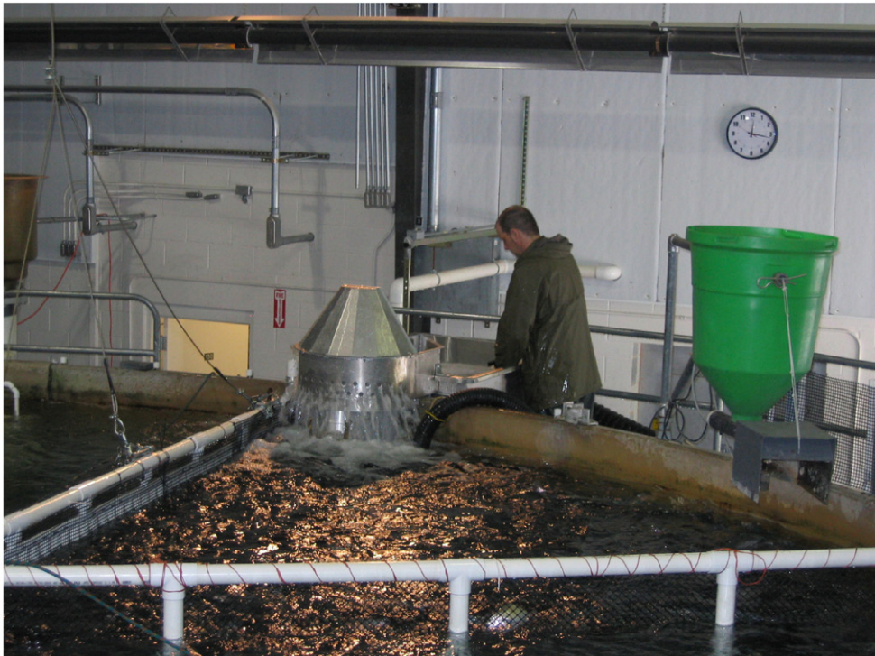
Fig. 11. Drawings (above) and photo (below) of a second airlift fish pump/dewatering/sorting box that was bolted to the wall of the culture tank and channeled the outlet water through the wall of the culture tank (drawings by Fabritek Inc., Winchester, VA).
