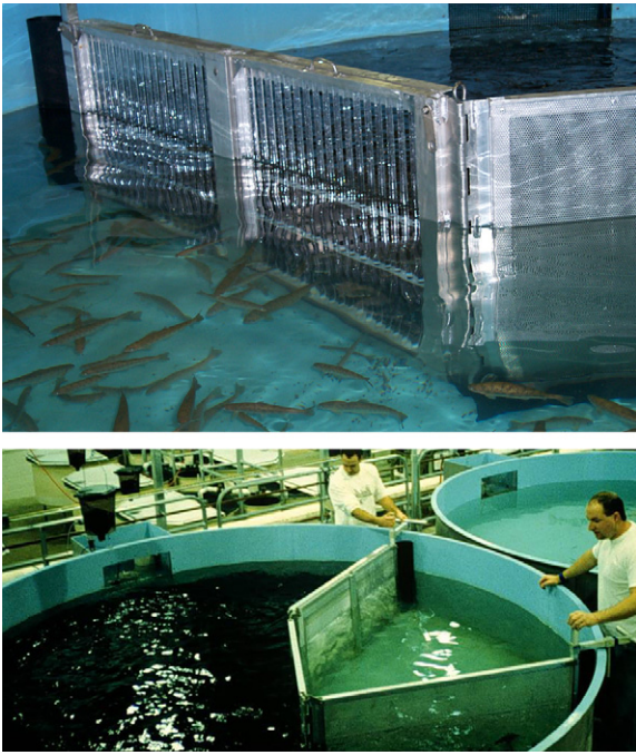
Fig. 6. A 3-panel clam-shell crowder/grader (Grade-Right™, Lance Industries, Bayboro, NC) has been used for over 8 years to crowd Arctic char or rainbow trout in the 3.7 m diameter by 1.1 m deep nursery tanks at the Conservation Fund Freshwater Institute. The fish crowded within the clam-shell grader were given up to 1 h to self-size sort as the smaller (less than 110 g) fish swam through the 1.91-cm (3/4 in.) gaps between the clear acrylic bars and into the open part of the culture tank.
