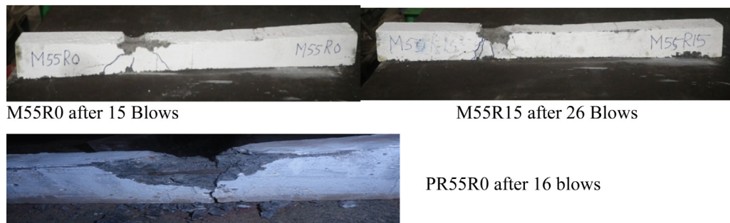
Figure 3 Crack pattern of ordinary, rubber and prestressed concrete.
