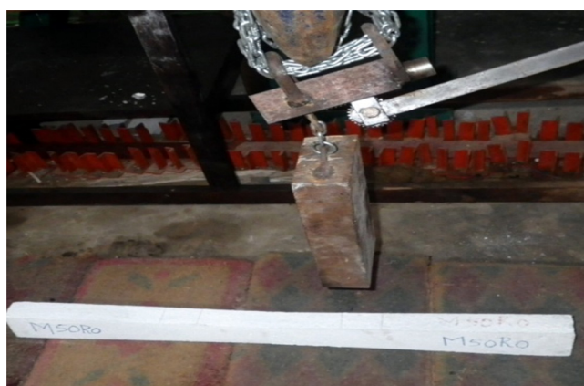
Figure 2 Test setup for impact test on railway sleeper.
