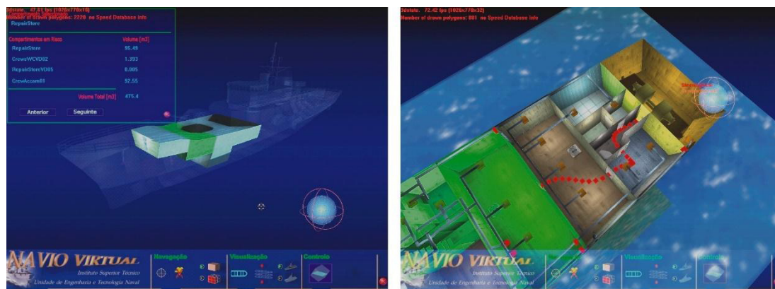
Figure 4: Zones with risk of flooding may be identified based on the current ship condition. Compartments are highlighted and the operator gets an initial estimation of the total zone that is in risk. Then, evacuation paths may be created between two compartments based on the current ship condition and concerning the risk zones that may exist along the way.
