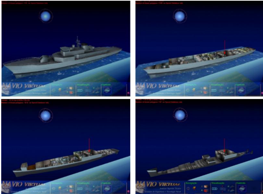
Figure 3: The deck-based visualization approach allows to observe lower decks by hiding the upper ones.
