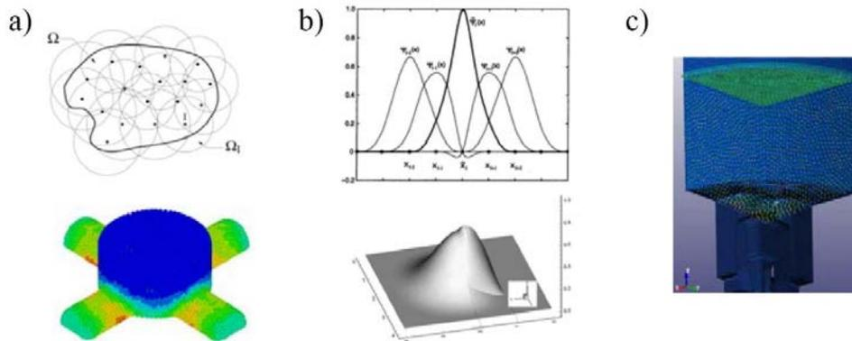
Fig. 1 (a) sub-domains definition, nodes 3D representation; (b) Spline kernel functions for EFG; (c) EFG numerical model.
