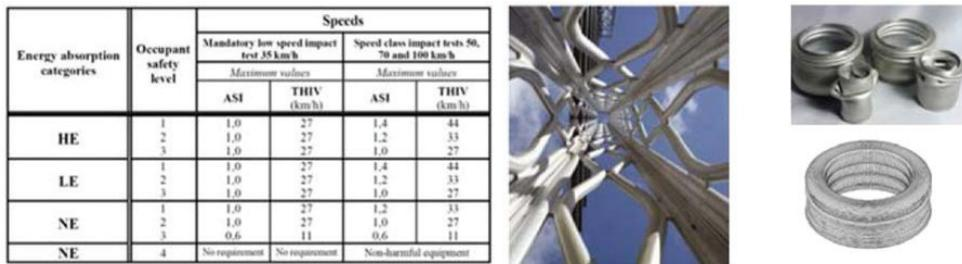
Fig. 2. European standard EN 12767, 2007 energy absorption demands, aluminium gantry profiles and crash tests/simulation results.
