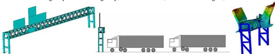
Fig. 5. Portal gantry model, vehicle tuned passage scenario and its resulting deflection.
