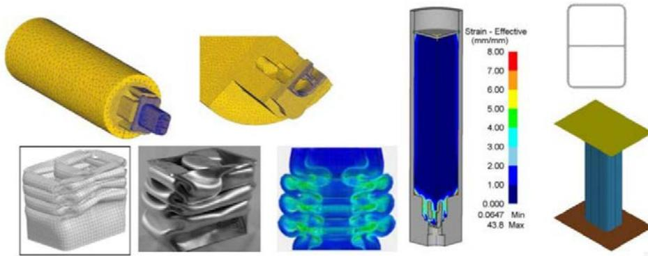
Fig. 6. FE mesh, effective strain contours, crash experimental test results along with simulated folding results.
