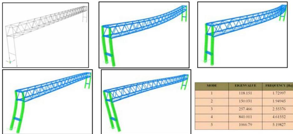
Fig. 4. Portal gantry line element model, its first four mode shapes and natural frequency table.
