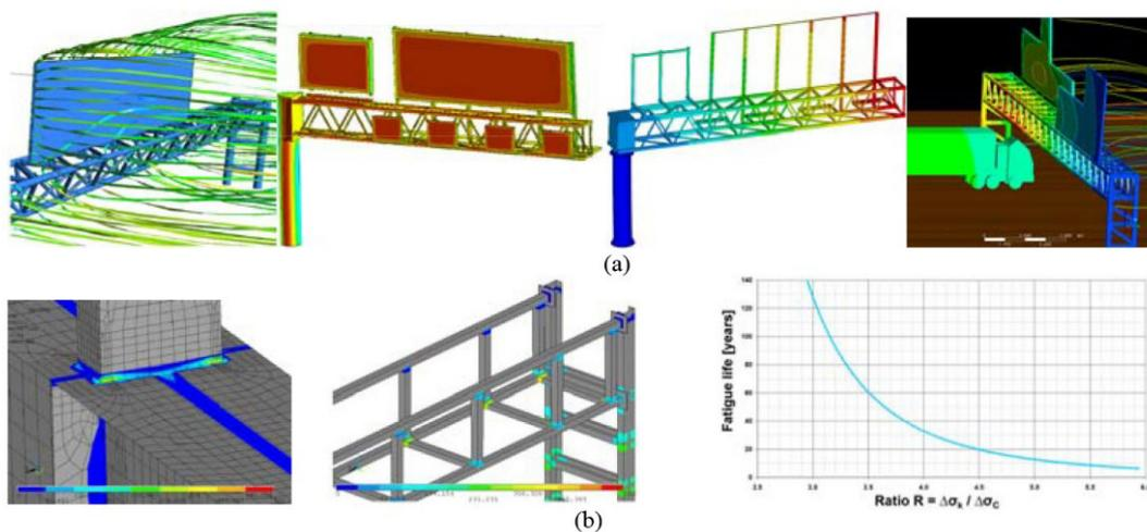
Fig. 3 (a) Gantry structures in virtual wind tunnel (environmental and vehicle buffeting); (b) Contour of fatigue life for critical gantry joints and automated fatigue life assessment graph.
