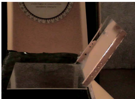
Figure 1. The dedicated cassette holder made from perspex is shown on the treatment couch.
