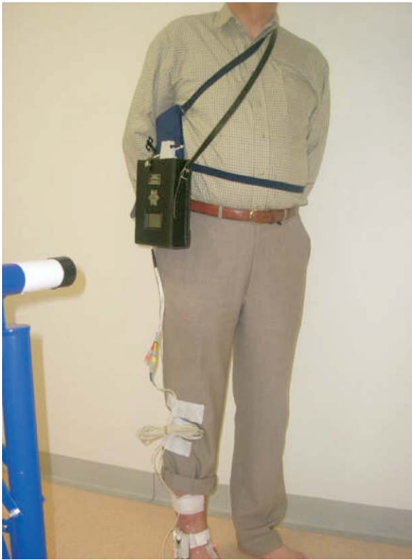
Fig 2. The continuous ambulatory venous pressure monitoring data logger (black bag) and syringe driver (blue bag) fitted to a patient. It allows full mobility during continuous pressure measurement.
