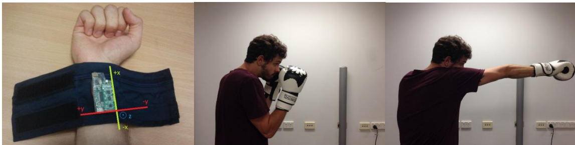
Figure 1: The acceleration sensor is fixed to the inside of the wrist with a velcro band. The boxing glove covers the sensor. (a) Sensor position and axis definition, (b) guard position of the boxer (c) full extension of the lead hand for a punch.
