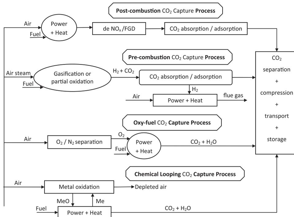
**Fig. 1.** CO<sub>2</sub> capture technologies.
