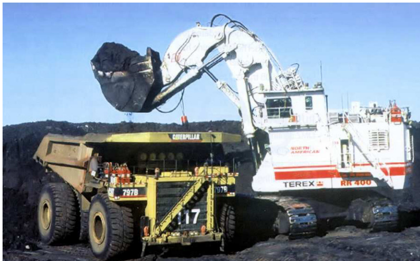
Fig. 6. Truck sizes can be up to 400 tonnes and shovel sizes, up to 80 tonnes
