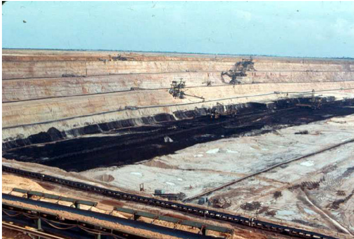
Fig. 5. A large continuous surface mine with bucket wheel excavators in the overburden [60 m thick] and the ore body [20 m thick]
