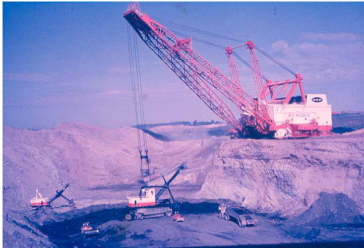
Fig. 4.A dragline in a strip coal mine. Draglines have bucket capacities of 140 \text{ m}^3 and reach of up to 90 m. Notice the two loading shovels and the trucks in the pit for ore handling.
