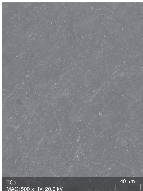
Fig. 4 – SEM microphotograph of a specimen of group TC (500x).
