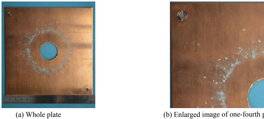
Fig. 5 Observation of craters due to ejecta impact on witness plates (Projectile of 3.2 mm in diameter, impact velocity 4.88 km/s).
