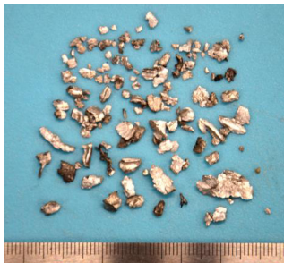
Fig. 3. Photograph of ejecta collected from test chamber (Projectile of 7.0 mm in diameter, impact velocity 3.57 km/s).
