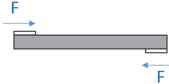
Fig. 7. Situation of forces applied to a cell in the string in the simplified model
