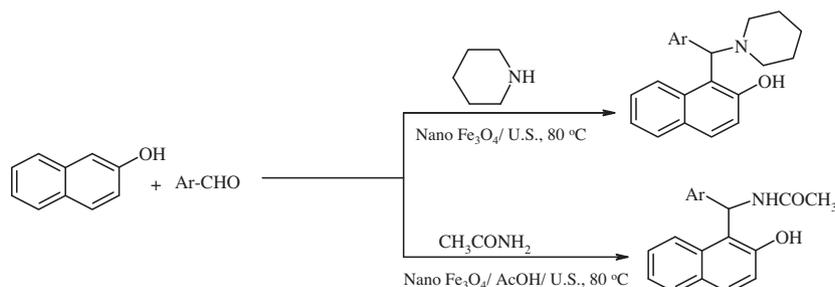
**Scheme 1** Fe<sub>3</sub>O<sub>4</sub> nanoparticle catalyzed synthesis of functionalized 2-naphthols.
