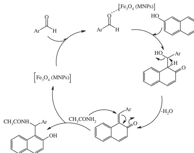
**Scheme 3** A plausible mechanism for the synthesis of *N*-((2-hydroxynaphthalene-1-yl)(aryl)methyl)acetamide derivatives.
