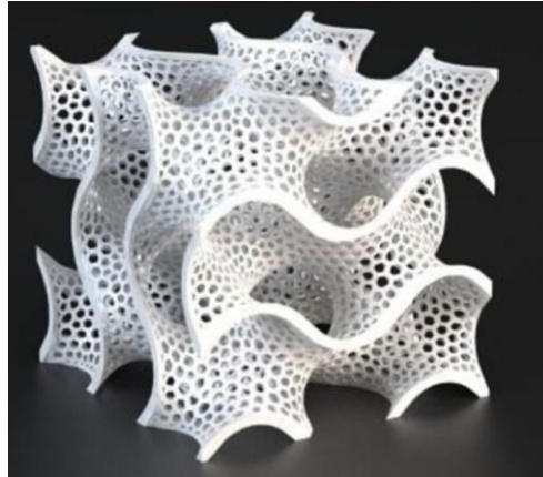
Fig. 4. Examples of parts made by SLS method [20].
