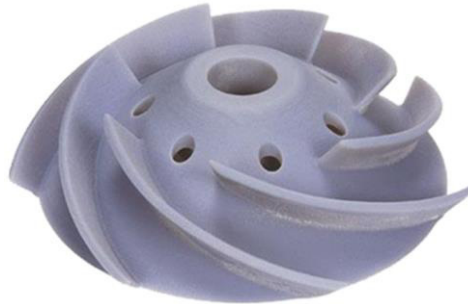
Fig. 6. Examples of parts made by PolyJet methods [26].
