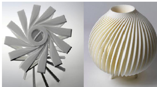
Fig. 7. Examples of complex shapes made by the method 3DP [28]
