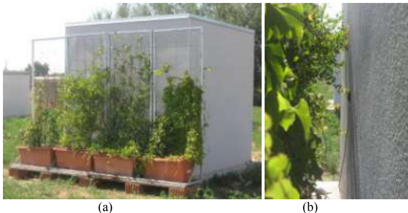
Fig. 3. (a) Cubicle with previous façade system; (b) free space between wall and green curtain
