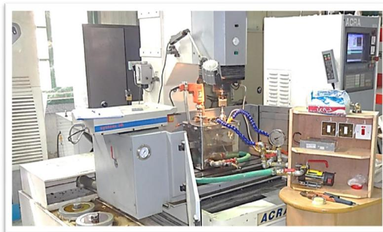
**Fig. 2.** The (CNC) EDM machine with all the fabricated accessories.
