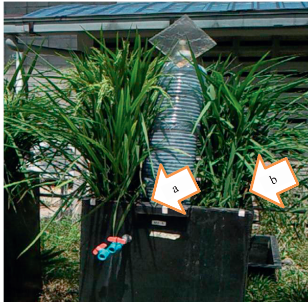
Fig. 1. A static chamber with a gas bag at 71 days after transplanting in MC1, also, some equipment relating to water level adjustment system has been shown in the picture (e.g. Adjustment valves in the front of the experimental plot (a) and the reservoir at the back (b))
