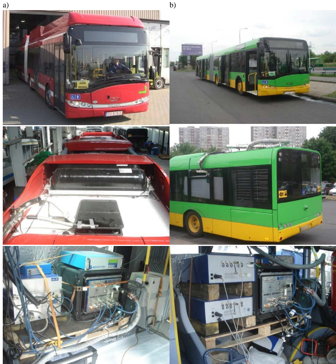
Fig. 2. Public buses with a length of 18 meters being prepared for the test: (a) a vehicle fuelled by CNG; (b) a vehicle fuelled by diesel oil.
