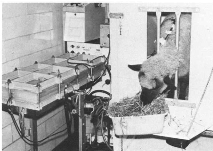
Fig. 1. Sheep being dialyzed while in a metabolic cage. The animal is retained in a stanchion, can stand or lie during dialysis, and can eat ad libitum.
