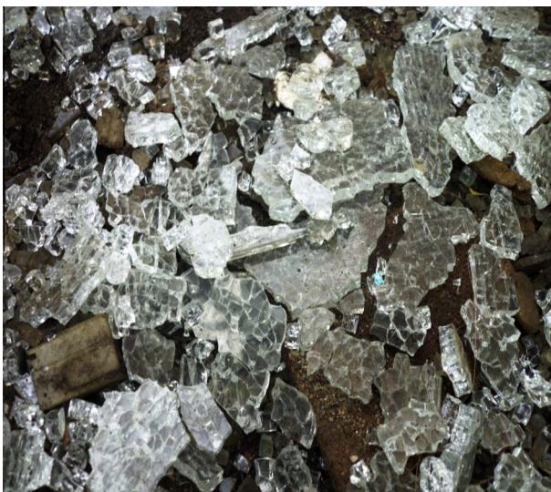
Fig. 1 – Fragmented car windscreen in a mechanic workshop.
