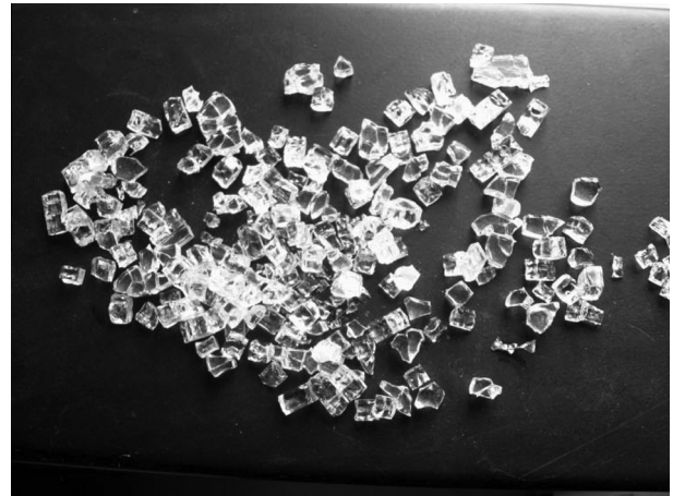
Fig. 2 – Separated washed glass beads.
