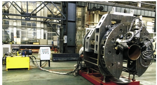
Fig. 13. On-land testing system for the multifunctional pipeline repair machinery.
