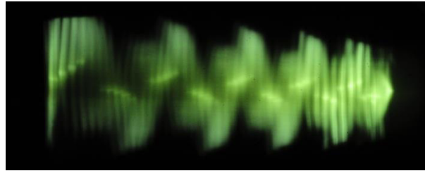
Fig. 3. Demonstration of radial betatron motion leading to increased turn-to-turn spacing at large radii noted at image right.
