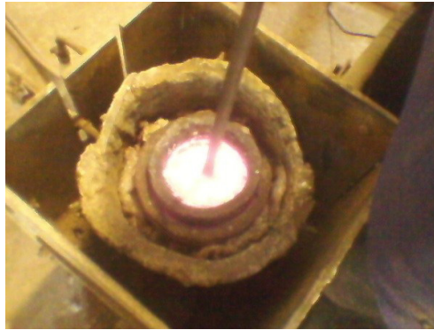
Fig.1 Molten metal in the furnace
