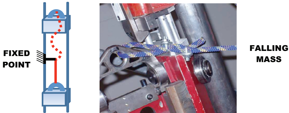
FIG. 1 The experimental apparatus (schematic) and a detail of the rope-mass connection (two clamps)
