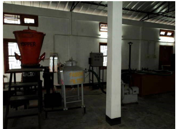
Fig. 5. Downdraft gasifier experimental setup
