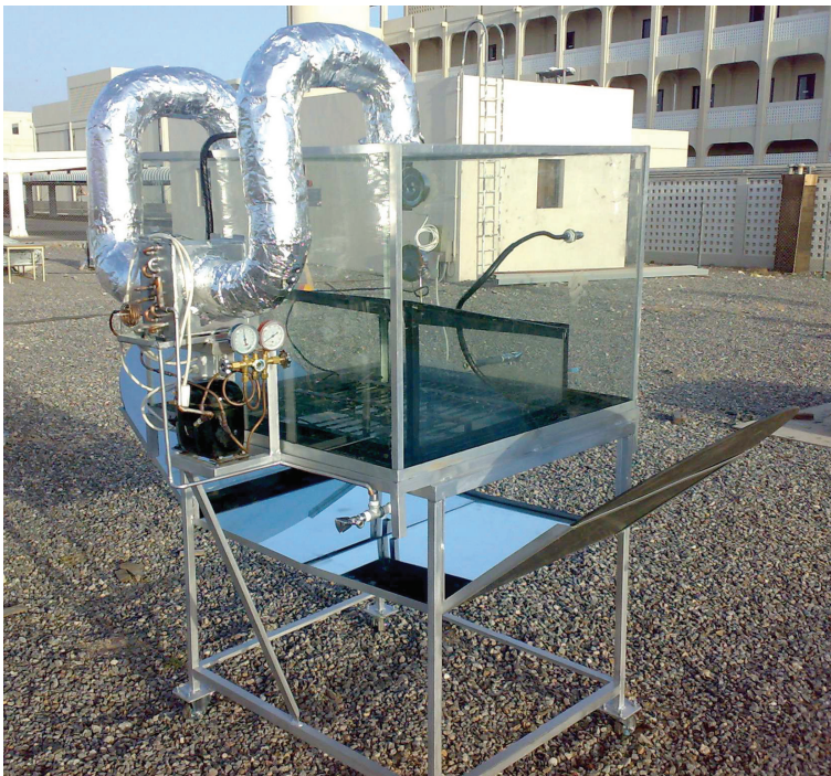
Fig. 2. Photographs of the refrigerated inverted solar still taken
