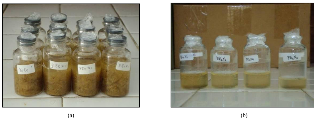
Fig 1. (a) The SSF process of sugarcane; (b) The ethanol of SSF results
