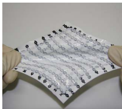
Fig.6: The stretchable active matrix did not exhibit any significant change in electronic performance even when it was stretched up to 80%
