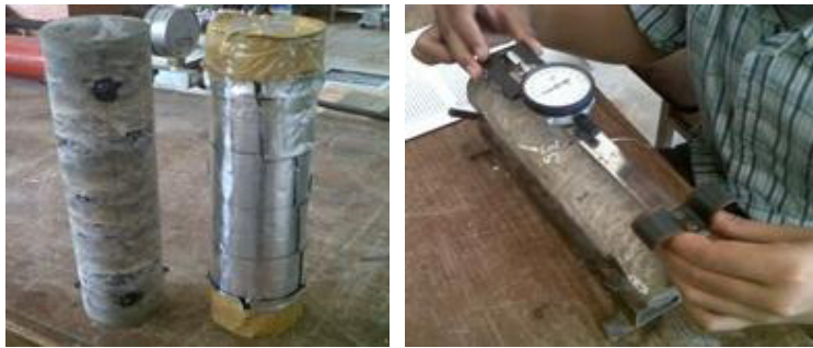
Fig.1. Unsealed and sealed specimens (left) and measurement of length change using Demec Gauge (right)
