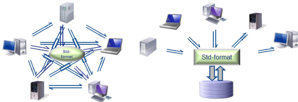
Fig. 3. Separate systems joined point to point (left) or via information hub (right) (Hallberg and Tarandi, 2011)
