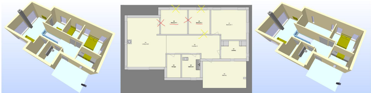
Fig. 6. The floor to export as IFC-objects in the Hub, the planned changes to do in Revit and the consolidated floor in the Hub
