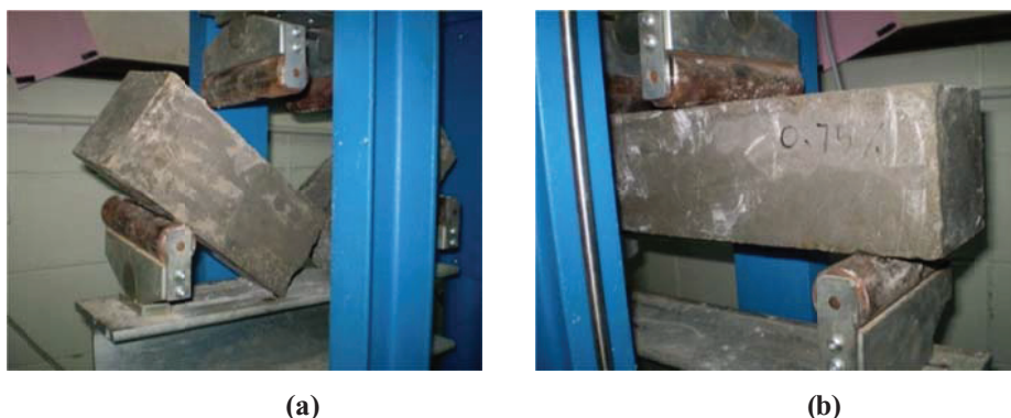
Figure 6: Flexural failure of beams: (a) Plain concrete, and (b) SFRC with 0.75% volumetric percentage
