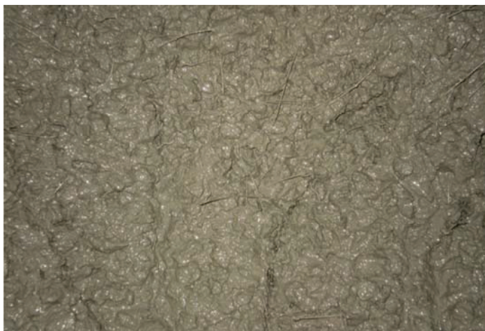
Figure 3: Physical appearance of fresh SFRC in the drum mixer
