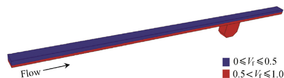
Fig. 8. Contours of volume fraction of water and air for X = 9 cm, U = 1.0 m/s, and d = 3.0 cm.
