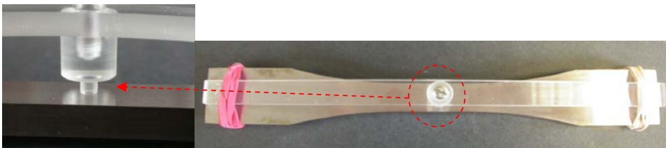
Fig. 1. Crevice former together with fatigue specimen
