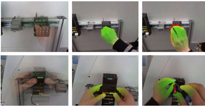
Fig. 38. Examples from an automatically authored AR-manual: the half-transparent overlays (left) were automatically extracted from the reference sequence. The green colouring (middle) indicates a correct completion of the task, red a wrong posture or position. [133].
