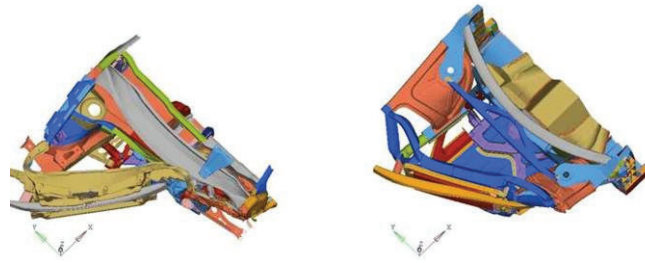
Fig. 104. Comparison of the reference's crash properties (left) with those of the developed front end (right)
