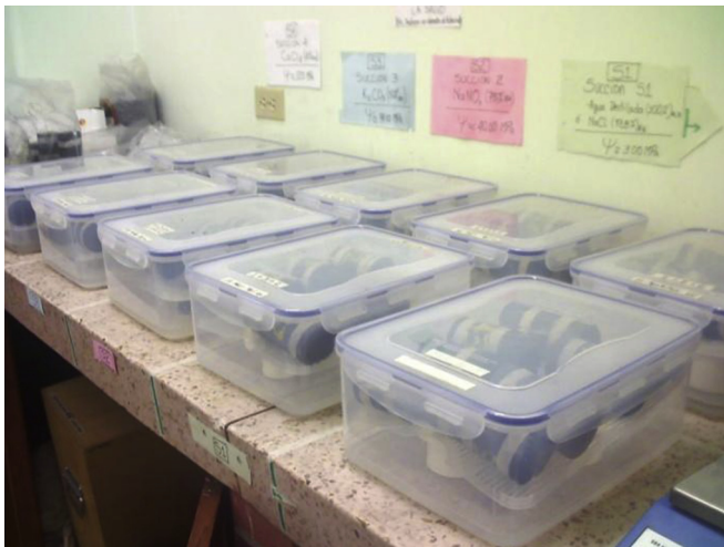
Fig. 5. Samples during suction cycles imposed by the VET.
