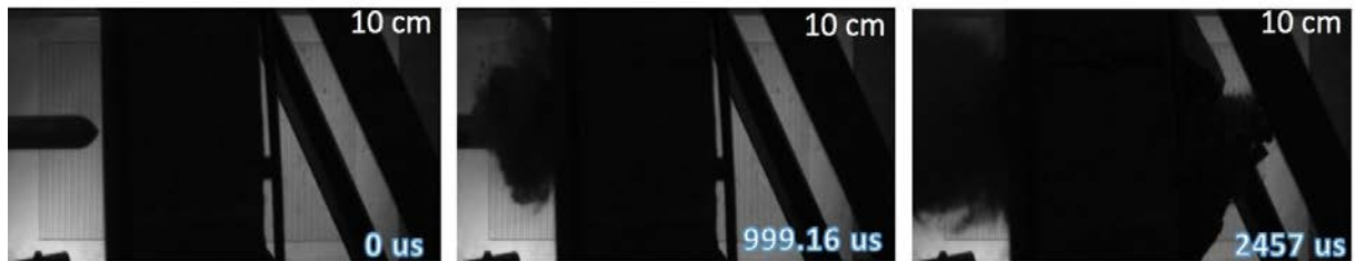
Fig. 5b. perforation process of 100mm thick concrete plate impacted by 1 kg steel projectile
