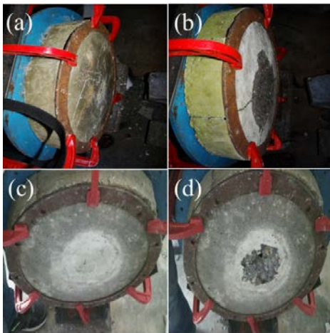
Fig. 3. 80 mm thick (a) and (b) plain concrete target and (c) and (d) reinforced concrete
