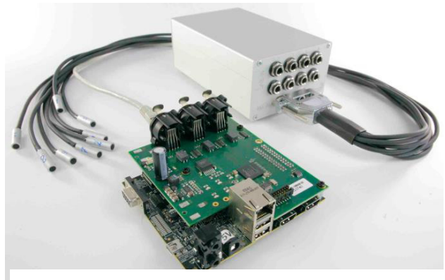
Figure 1 - Embedded acoustic processing unit together with audio satellite unit and 8 microphones.
