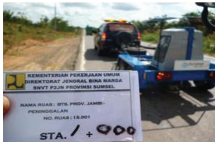
Fig.2. Falling Weight Deflectometer Measurement to collect pavement data
