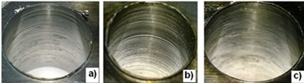
Fig 10 Images of Burr formation under different cutting speed.
