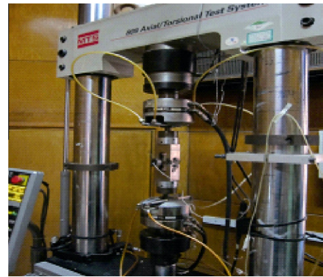
Fig. 3 Scheme of fatigue crack growth test.
